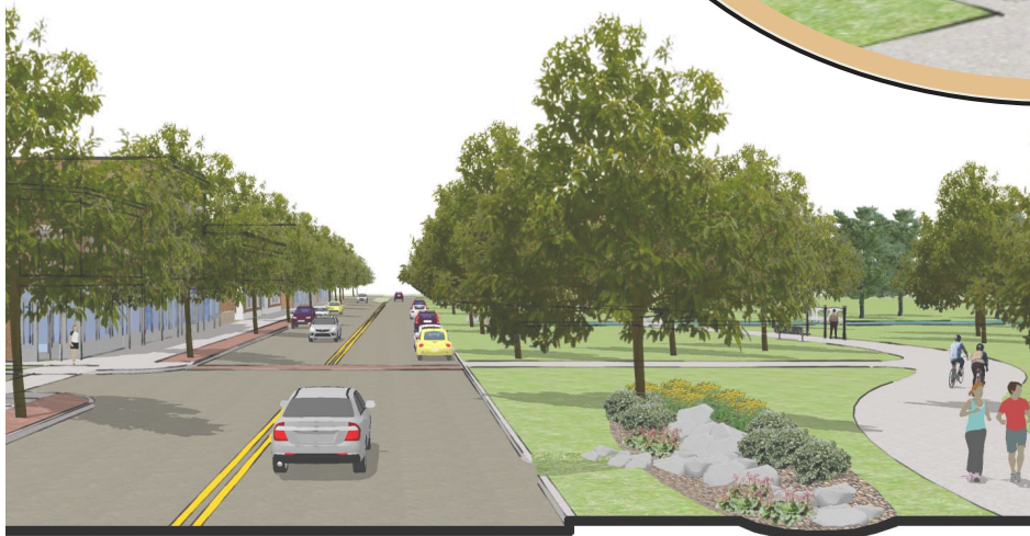
Illustration of the elements that make-up a Green Street
