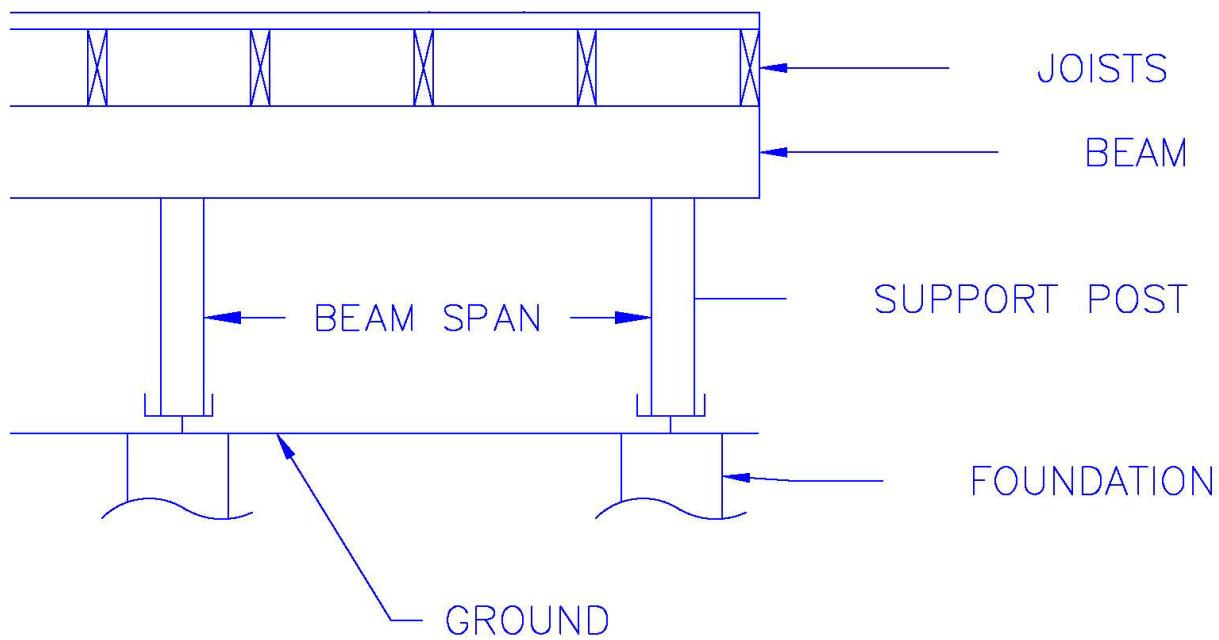
The span for the deck is:
