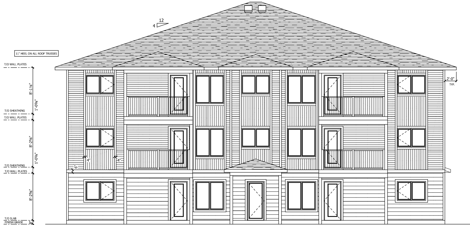
1 FRONT ELEVATION - TOP OF WINDOWS TO MATCH HEIGHT OF DOORS U.N.D. - 4" TRIM AROUND ALL WINDOWS AND DOORS AS SHOWN
