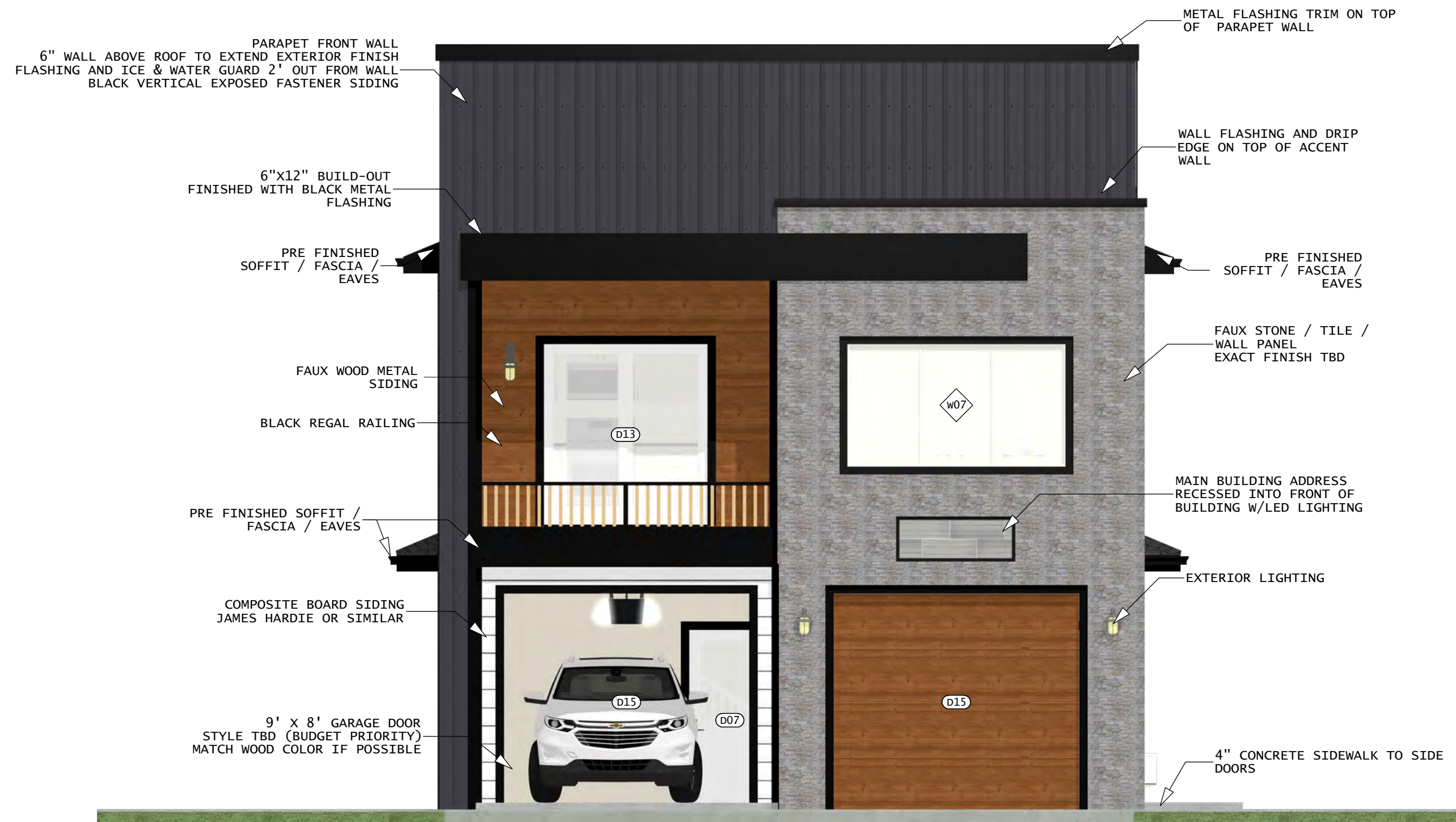
(E1) Exterior Elevation Front 1/4 in = 1 ft
