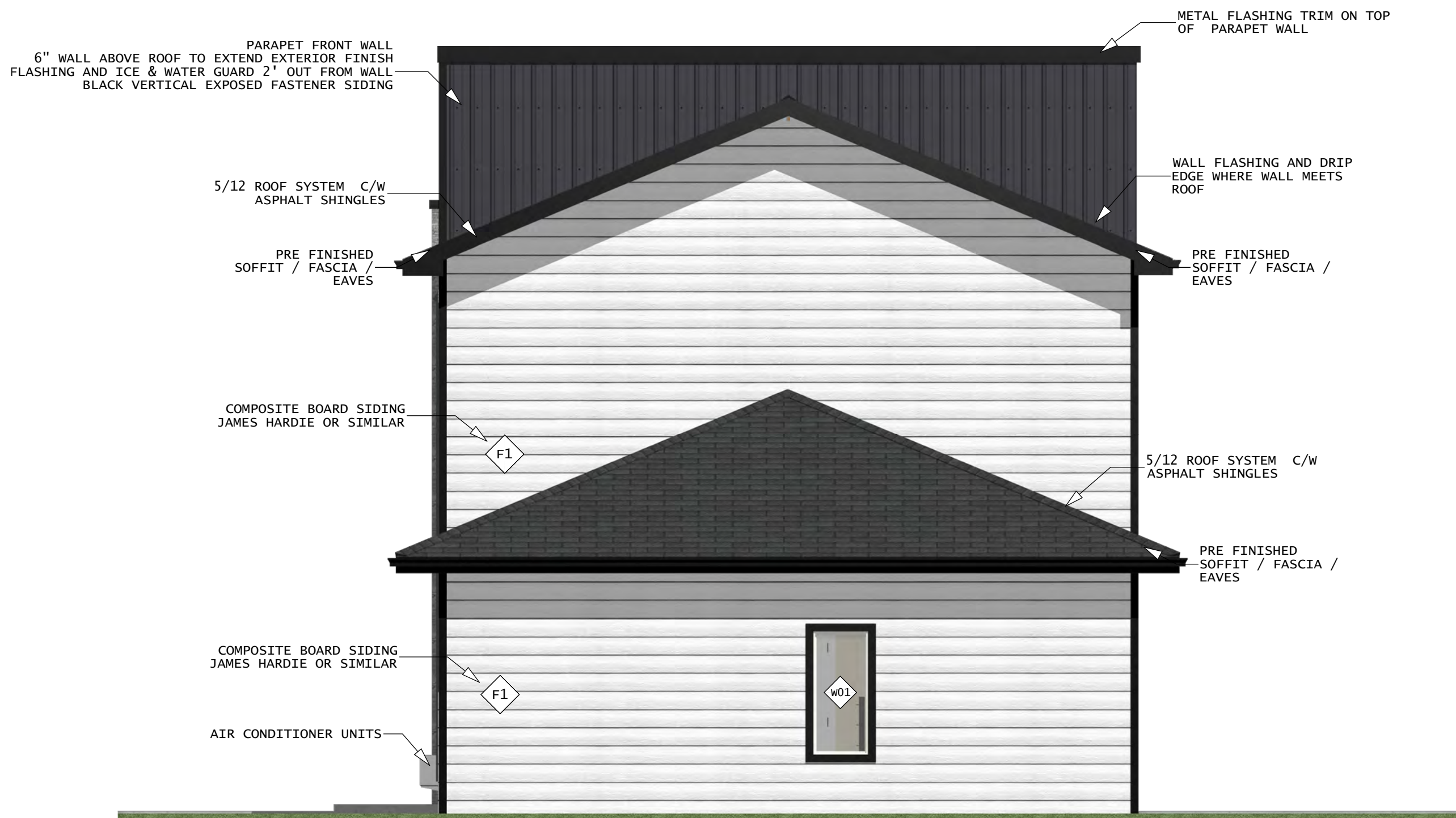
(E3) Exterior Elevation Back 1/4 in = 1 ft
