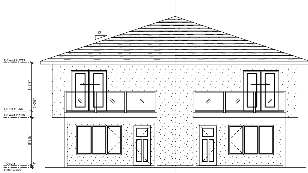
1 FRONT ELEVATION - TOP OF WINDOWS TO MATCH HEIGHT OF DOORS U.M.O. - STUCCO FRONT AND REAR - VINYL SIDING ON BOTH SIDES
