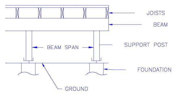
The span for the deck is:
